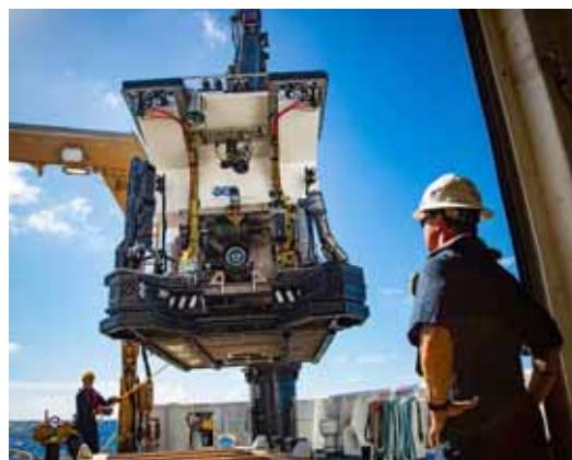
NOAA’s ROV Deep Discoverer (D2), conducted daily dives from 250 to 6,000 meters on the 2016 Deep-water Exploration of the Marianas. Photo: <http://bit.ly/2dKKxD5>, credit NOAA
