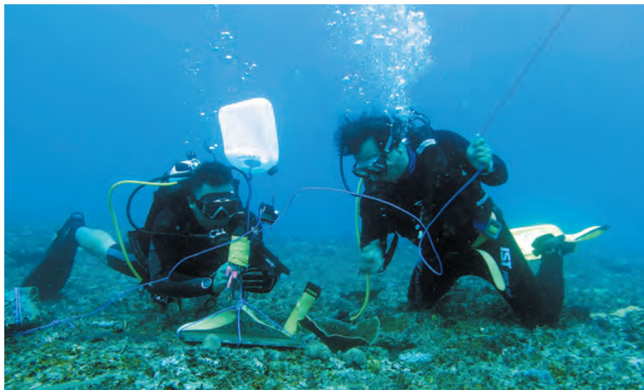
Researchers install hydrophones off the coast of Bali to measure the effect of Nyepi, a day of silence.
