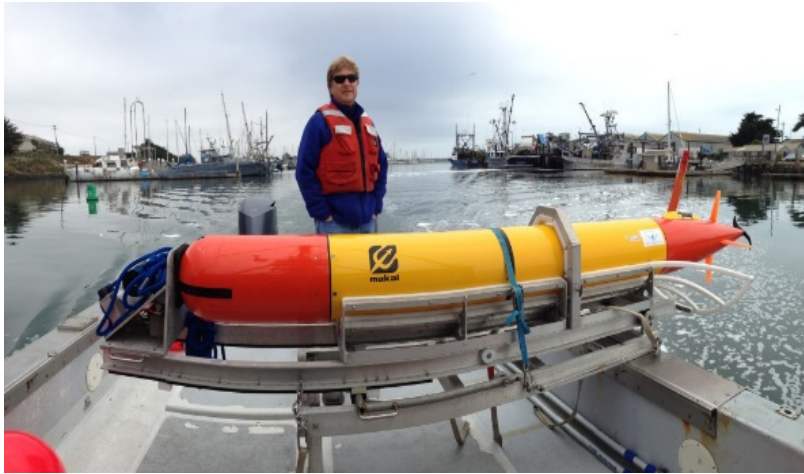
Figure 5. The MBARI Environmental Sample Processor (ESP), heads out to sea for the launch of a long-range autonomous underwater vehicle carrying the latest version of the instrument. Photo: Todd Walsh © MBARI 2017
