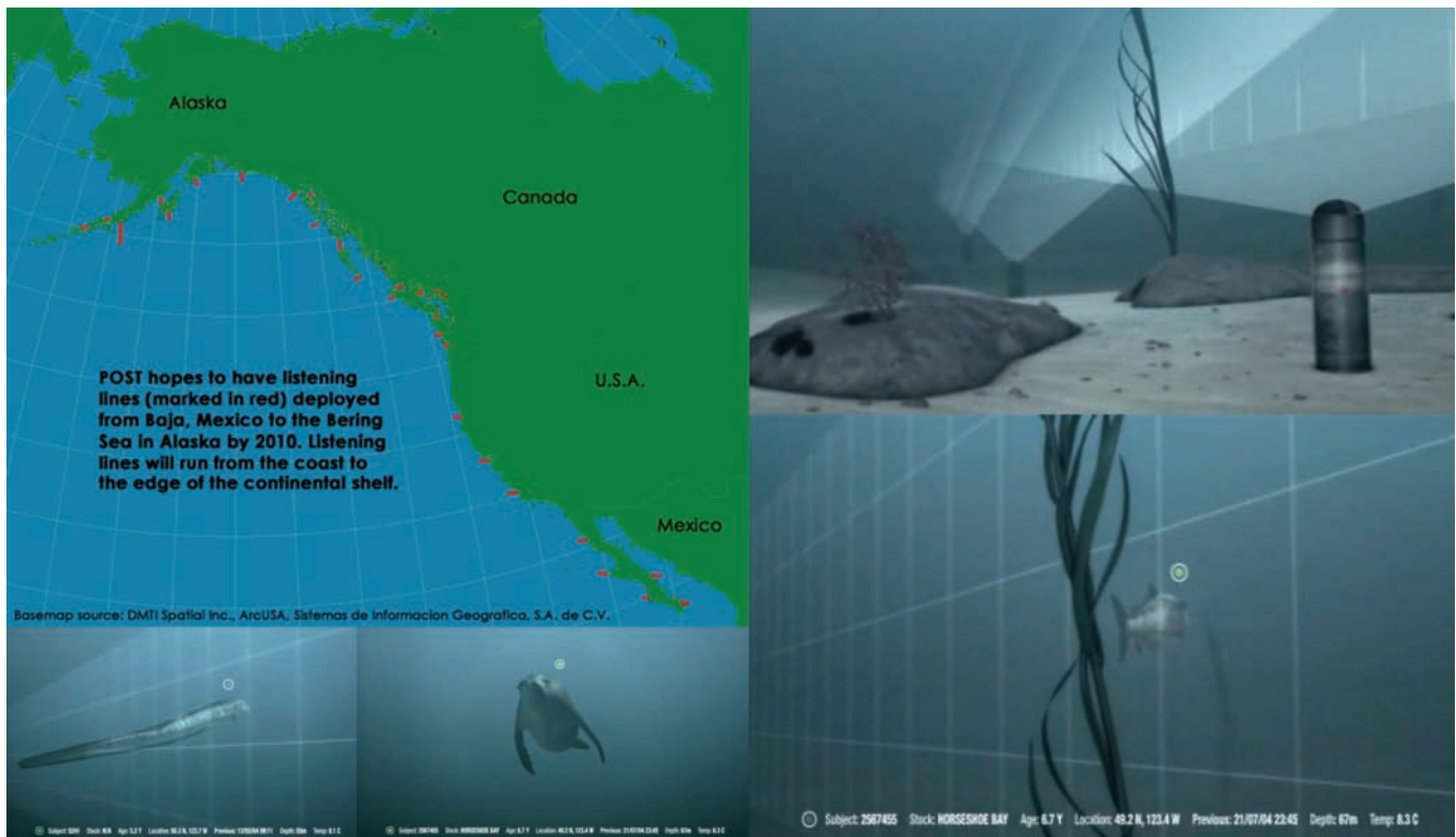
Figure 30. The Census of Marine Life Pacific Ocean Shelf Tracking (POST) project demonstrated the use of tiny coded acoustic tags to monitor movements of marine animals from juvenile salmon to herring, sturgeon, and sharks using listening curtains across continental shelves. The technology can be used on a wide range of species and a large number of individuals with over 200,000 tag codes. Source: Census of Marine Life.
