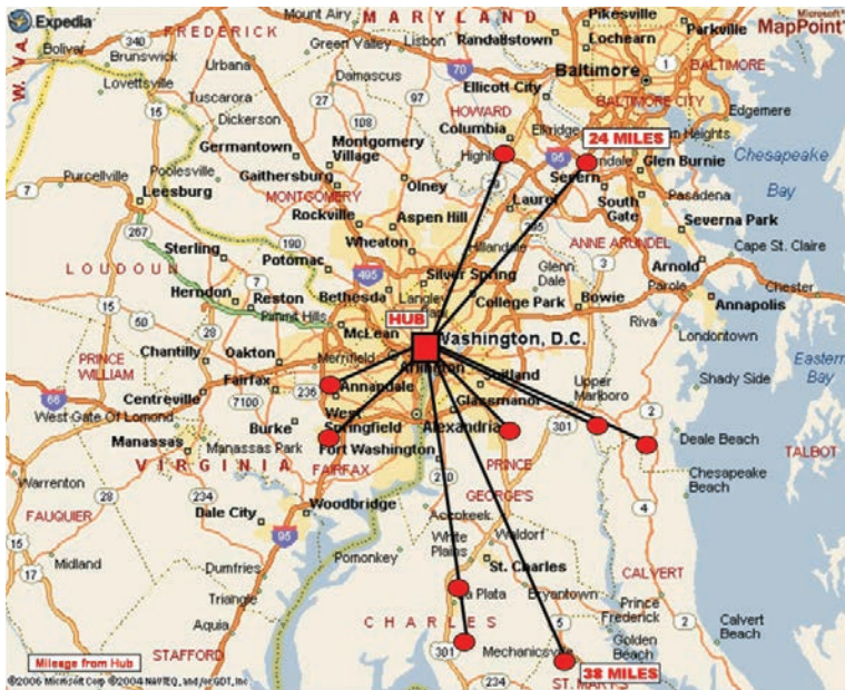
Figure 3. Gulf of Mexico Independence Hub's subsea reach superimposed on a map of Washington, D.C. Red circles indicate linked seafloor colonies of the square mother hub with a surface platform. These subsea tiebacks to a central control hub can be 40 miles long. Source: Thomas Fry, National Ocean Industries Association.
