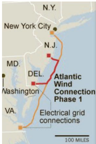
Figure 8. Google and a New York financial firm have proposed building a 350-mile underwater transmission line that could carry as much as 6,000 megawatts of electricity from wind farms off the mid-Atlantic coast. Source: New York Times, 12 October 2010.
