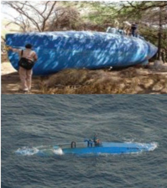
Figure 34. This semi-submersible, built in South America, has been fitted to transport up to 10 tons of illegal drugs to the United States. The virtually nonexistent freeboard makes them difficult to detect with radar and visually. The next step is complete submersion. Sources: Wikimedia Commons, globalsecurity.org.
